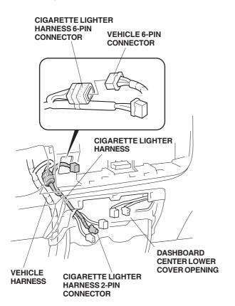
12. Connect the vehicle 2-pin connector and cigarette lighter harness 2-pin connector into the cigarette lighter socket. Reinstall the dashboard center lower cover.
