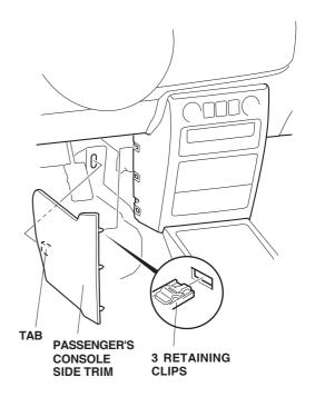
4. Remove the passenger's console side trim (two retaining clips and one tab).
